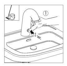
This will turn the water off for approximately 75 seconds so that the sink may be cleaned (2).
